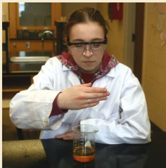
Figure 1.3 Never smell anything in the lab directly. Always waft the fumes toward your nose.
